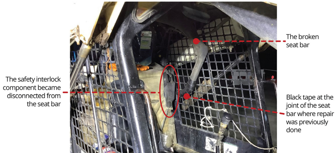
Figure 2: The skid-steer loader's seat bar broke at a location which made the safety interlock ineffective.
